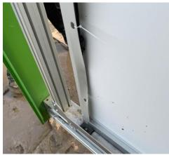
Figure 20 Transport damage
